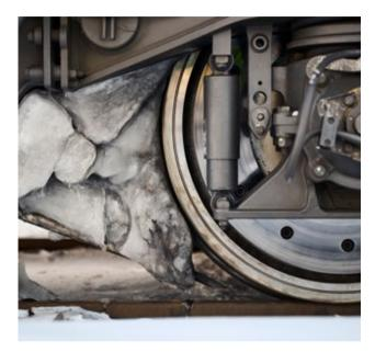
It can be challenging for wheels and brakes when the blue ice starts to stick.
